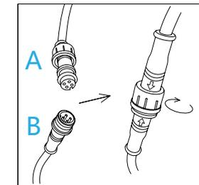
• Ensure the arrow icons are aligned on the two cables
