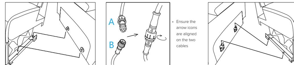
• Ensure the arrow icons are aligned on the two cables
